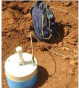
Figure 1. Field experiment with stalk seeds of sugarcane inoculated with diazotrophic bacteria. Blue tubes are the bases of chambers installed to allow the collection of green house gases, including  $N_2O$ , emitted from soil and N fertilizer. Gas sampling in the field
