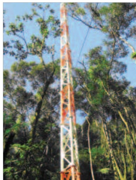
Micrometeorological Eddy Covariance flux tower installed at Núcleo Santa Virgínia/PESM, São Luis do Paraitinga/SP
