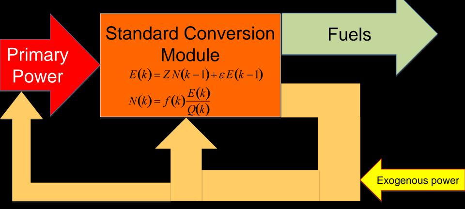
A fraction of the primary power converted by the module has to go back to supply power for growth, maintenance, replacements, and feedstock production. This fraction may exceed the total power generated by the module (exogenous growth).
