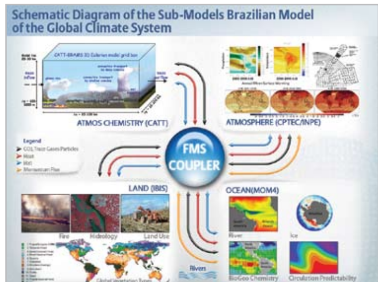
Figure 1. Schematic Diagram of the Brazilian Model of the Global Climate System and its sub-models. The four sub-models – Atmosphere, Atmospheric chemistry, Ocean and Land – are integrated by a coupler
