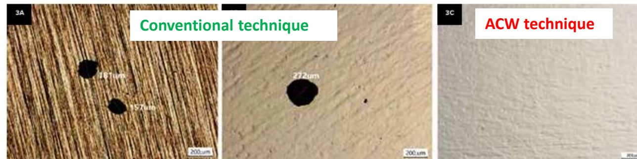
Figure 3: Optical micrographs of 316L stainless steel scanned surface area after CPP measurements of A: Ra = 0.8 μm grinded surface with E_{pit} = +365 mV; B: Ra = 0.3 μm electropolished surface with E_{pit} = +716 mV; and C: Ra = 0.3 μm electropolished and passivated surface without E_{pit} . Electrolyte: 3.5% (m/v) NaCl.
